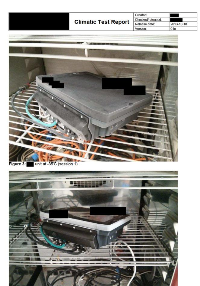
Figure 4: unit after loading from -35°C to +80°C (after se ssion 1)
